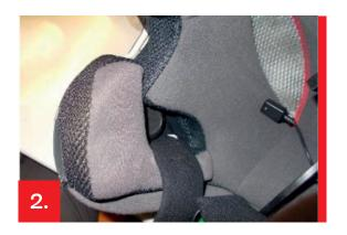
Place the right speaker (R) on the cheekpad's pp plate after applying the adhesive round shaped velcro included in the package.
