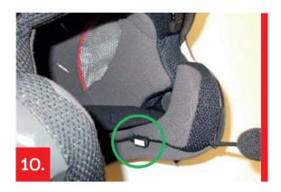
Place the USB socket between the cheekpad and the neckroll.
