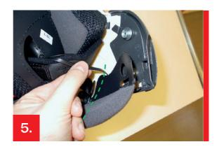
Pass the flat cable of the remote control cable between the neckroll's pp plate and the shell. The remote control must remain accessible outside the helmet.
