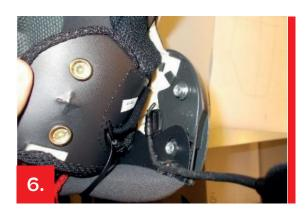
Place the base of the microphone under the cheekpads, place the microphone's boom in the seat ensuring that the neckroll pp plate has been previously positioned against the shell.
