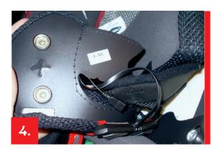
Without pulling the chinstrap out of the cheekpads, pass the microphone cable and the flat cable of the remote control into the hole of the cheekpads.
