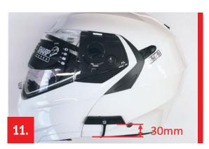
Fit the keypad on the left side (helmet on), approximately 30 mm from the lower edge of the shell using the provided adhesive. Make sure that there is no interference with the chin guard and full contact surface between the adhesive keypad and the outer shell.
