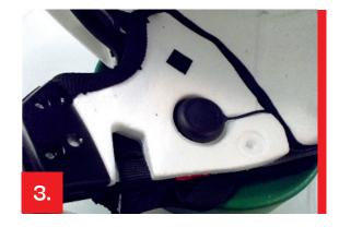
Place the right speaker (R) in its seat after applying the adhesive round shaped velcro included in the package.
