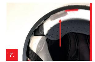
Place the BT controller in the designated slot on the back of the inner shell.
