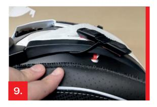
Pass the flat cable of the remote control between the neckroll's pp plate and the shell. The remote control must remain accessible outside the helmet.
