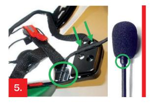
Place the microphone base under the chinstrap in the cavity of the EPS cheekpads. Fit the microphone boom in the seat in the inner plate
