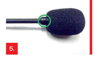
Adjust the microphone's position by deforming its boom.
