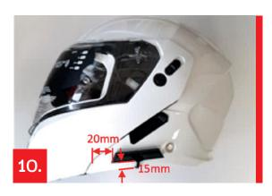
Fit the keypad on the left side (helmet on), approximately 15 mm from the lower edge of the shell using the provided adhesive. Make sure that there is no interference with the chin guard and full contact surface between the adhesive keypad and the outer shell.
