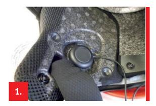
Remove the inner linings as indicated in the communicator's user manual.
