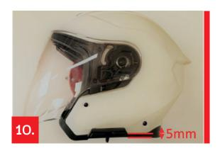
Fit the keypad on the left side (helmet on), approximately 5 mm from the lower edge of the shell using the provided adhesive. Make sure that there is no interference with the chin guard and full contact surface between the adhesive keypad and the outer shell.
