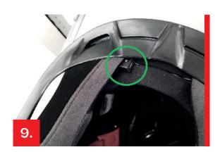
Place the USB socket between the inner linings and the shell.
