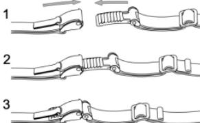
**SO ÖFFNEN UND LÖSEN SIE DEN MIKROMETRISCHEN RIEMEN**
