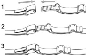
**HOE HET MICROMETRISCHE RIEMPJE OPENEN EN VERWIJDEREN**
